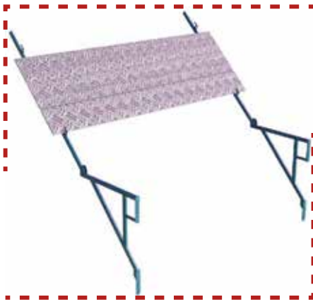
SCAFFOLDING FALL OF DEBRIS
